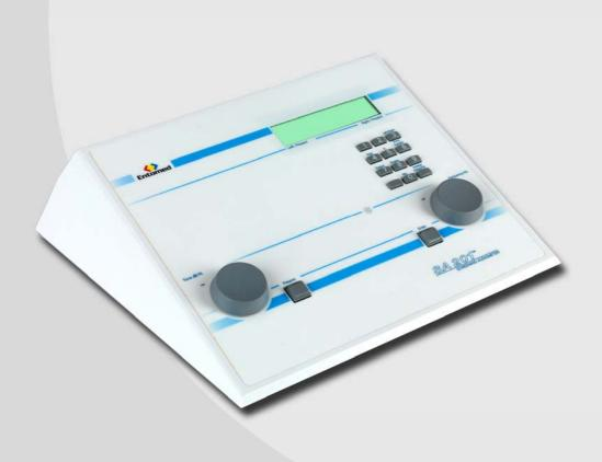
SA 201 is a basic, manual, two channel, pure tone air conduction, screening audiometer with full frequency and output range. SA 201 is digital and RoHS compatible and thus, well adapted to the modern user and environmental concerns. SA 201 is user friendly, robust, reliable and yet affordable.
