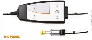
Clarinet features an extremely light, small and sturdy metal probe, which can be very rapidly disassembled and cleaned. The probe is connected to the small Control Box, through which you can select the ear and start the exam.
