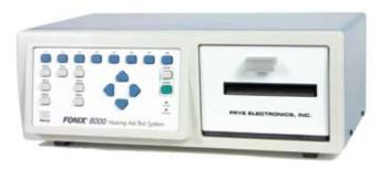
In the Input/Output test screen, you can measure the compression characteristics of the hearing aid at any frequency between 200 and 8000 Hz in 100 Hz intervals. Alternately, you can choose to use the broadband Composite signal.
